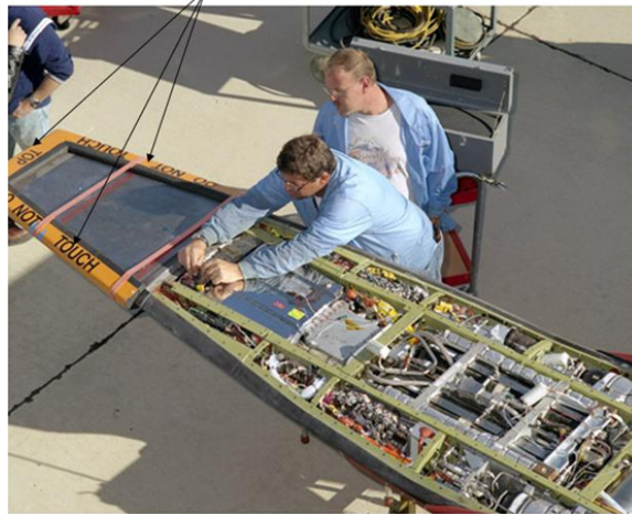
Figure 1. NASA technicians assemble the scramjet-powered X-43A Test Vehicle before its record Mach 9.6 Flight.
