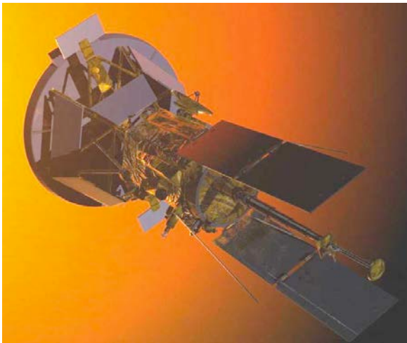
Figure 13: Solar Probe Plus, a (real) mission to the corona of the sun. The carbon heat shield protects the spacecraft from the high-intensity thermal environment of the sun.
